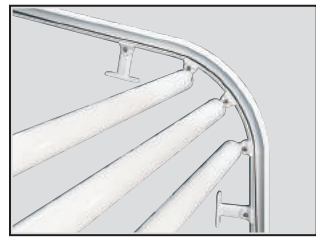
relieving rollers in the curved section
